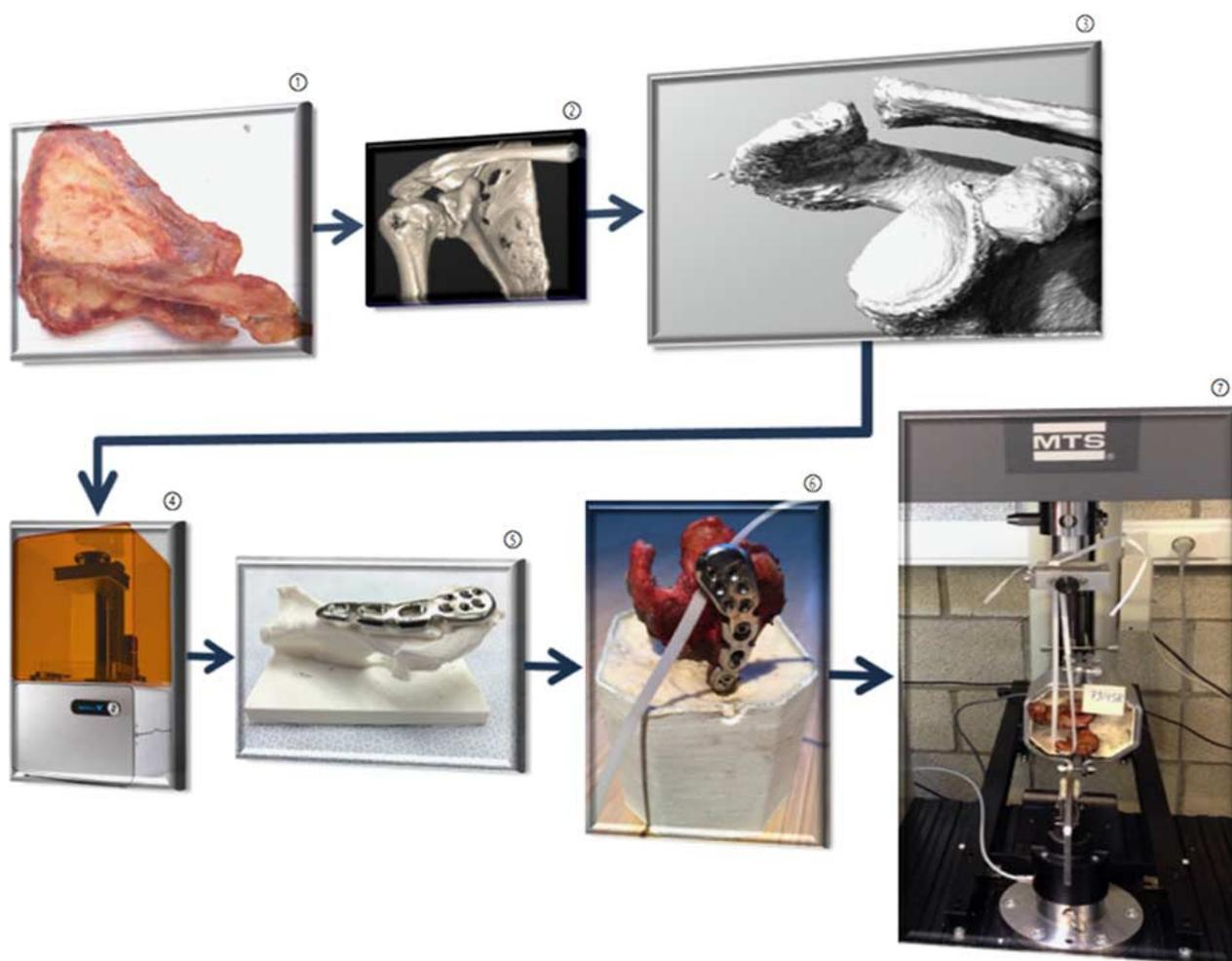
**FIGURE 1.** Study design. 1, Scapula of fresh-frozen cadavers. 2, Three-dimensional (3D) computed tomography scan according to a protocol. 3, A 3D processing: segmentation and digital planning to STL file. 4, A 3D printing. 5, A 3D model of patient-specific bended osteosynthesis plate. 6, Plate osteosynthesis technique. 7, Biomechanical testing. [full color online](#)
