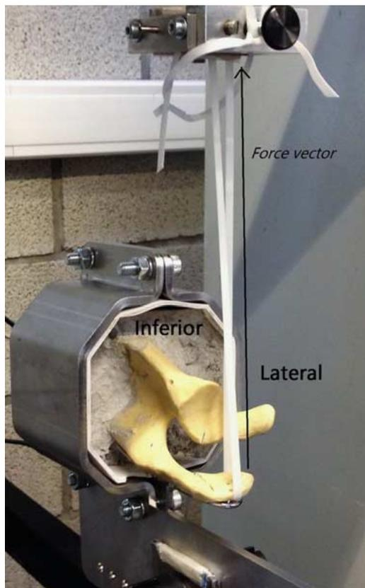
**FIGURE 3.** Test setup. A polypropylene rope was fixed in parallel to the dorsal acromion edge 1 cm from the anterior protrusion. The 2 ends were clamped and tied to the upper part of the testing machine. The force vector is parallel to the surface of the acromion. full color online
